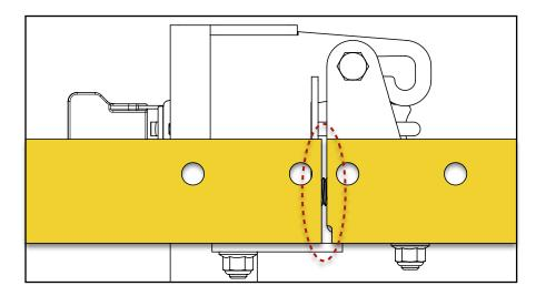
If the track rails are parallel but a gap still exists between the rail seam (while the latches are engaged), the rails can be brought together by loosening the bolts that secure the hinge bunk to the track rails.
