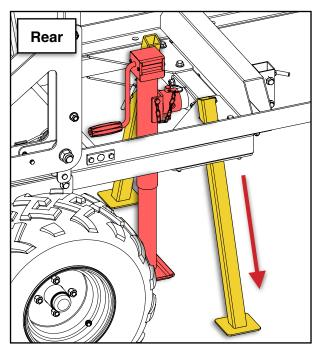
Once level, lower all the support legs and lock them in place with the T-bolts. Check the level of the track rails at the ends of the track and adjust the outer supports if necessary.
