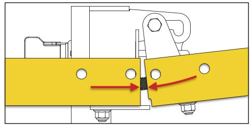
Loosen the jam nuts and use a hex key to adjust the two (2) set screws.
