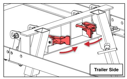
Disengage the two (2) hook latches by pulling the handles inward to release them.
