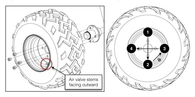
With the wheels mounted properly, the tread patterns should now be oriented as shown below.
