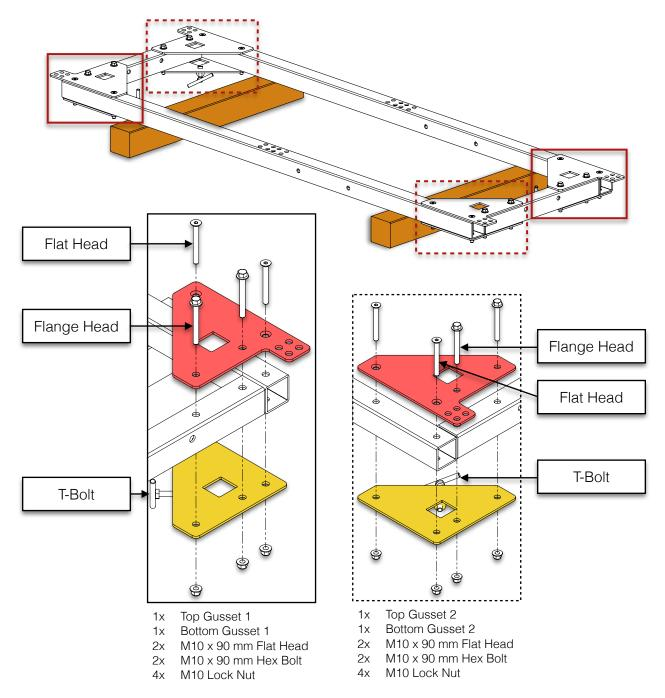
Assemble the trailer box frame on wood blocks for ease of assembly. The diagonally opposite corners are the same. Note that the two (2) flat head screws in each corner are assembled through the countersunk holes.
