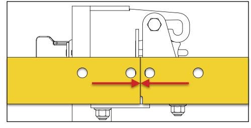
Re-latch the two (2) hook latches to pull the track rails together and then check the fit.
