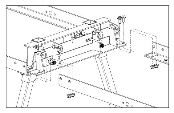
If the top faces of the track rails on the extension aren't collinear with track rails on the main trailer, the provided shims can be used between the hinge bunk flanges and track rails to bring them in line. This step is not necessary if the rails are already inline.
