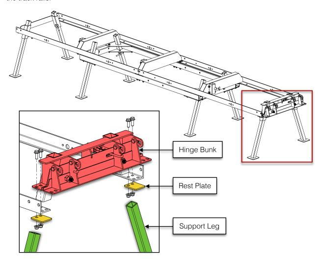
Continue with the trailer assembly after the hinge bunk is installed.
