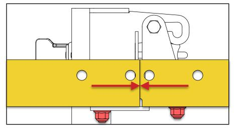
After the track rails are pulled together, retighten the hinge bunk bolts.
