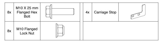
Note that the carriage stops are assembled to the *inside* face of the track rail.
