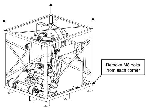
Remove all the loose components from the skid (infeed chute panels, control arm, edge bar, control arm linkage, discharge chute, discharge chute handles, PTO shaft) and set them to the side. Leave the wood chipper on the skid.
