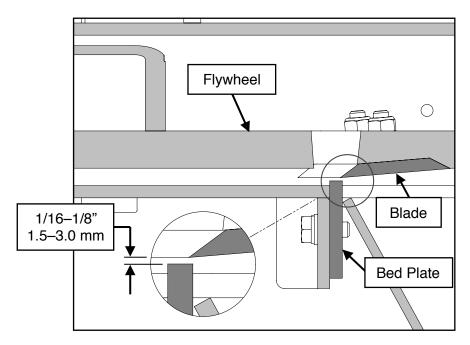
4. Use a socket/wrench to loosen the three (3) M10 X 25 mm hex bolts securing the bed plate to the lower flywheel housing so the bed plate is free to slide in and out. This movement will increase or decrease the gap between the bed plate and the cutting edge of the blade. Slide the bed plate by gripping the knob and adjust its position so that it is within 1/16-1/8" (1.5-3.0 mm) of the cutting edge of the blade. Ensure the gap is uniform along the entire edge of the blade.
