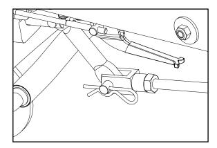
Once the linkage has been assembled, use a wrench to ensure both M10 jam nuts are tight.
