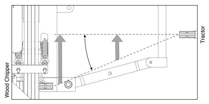
4. Measure the straight-line distance between the locking grooves on the splined shafts of the tractor and wood chipper (**Dim A** below).
