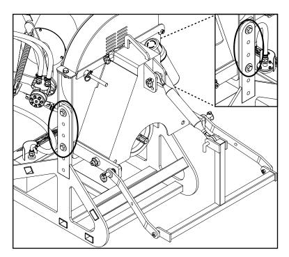
Reattach the base to the housing using the four (4) M16 X 60 mm hex bolts and M16 X 45 mm fender washers. Secure the bottom two (2) bolts with the M16 lock nuts.
