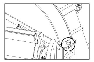
3. With the flywheel exposed, manually rotate it so that one of the four (4) locking holes in the flywheel (near the front of the blade) approximately lines up with the flywheel lock pin at the rear of the housing. Remove the small locking pin from the flywheel lock pin and flip the flywheel lock pin around 180°, passing it through the housing and into the locking hole in the flywheel. Reinstall the smaller locking pin to the flywheel lock pin.
