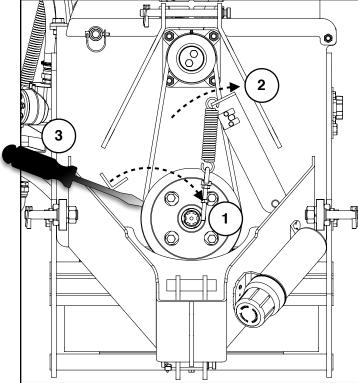
With the eyebolts disconnected from the bracket, let them hang loose from the springs while still attached to the tension arm<sup>1</sup>.
