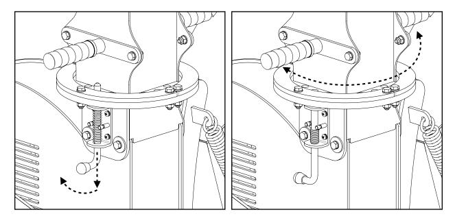
The chip deflector easily adjusts to regulate the distance the chips are thrown. Rotate the handle counterclockwise to loosen the deflector, adjust the deflector to the desired angle, then re-tighten the handle by rotating it clockwise to secure the deflector.
