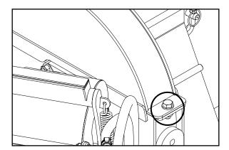
3. With the flywheel exposed, manually rotate it so that the first blade lines up with the bed plate and note the gap between them. Use a flash light for better viewing if necessary. Repeat this process for the remaining three blades, noting which blade is closest. Use this blade to set the bed plate gap.
