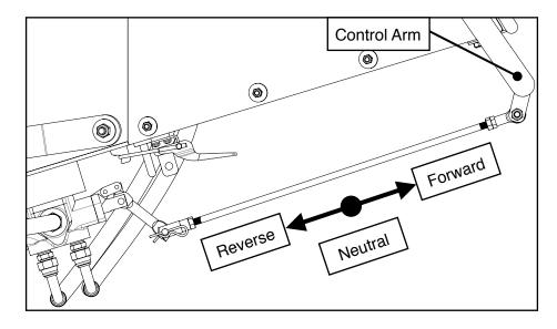
To change the speed of the infeed roller, place the red control arm in the *neutral* position. This stops the infeed roller from rotating. The speed control valve can now be moved to the desired position/speed. Reengage the infeed roller via the control arm.
